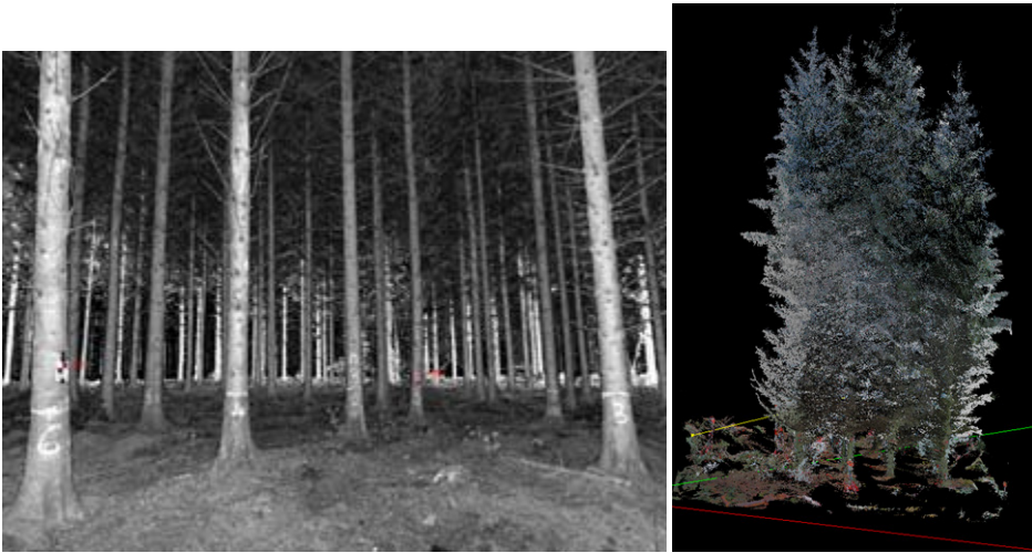
Fig. 7. Below-canopy plot sampling using terrestrial laser scanning. Images courtesy of Forest Research, UK.
